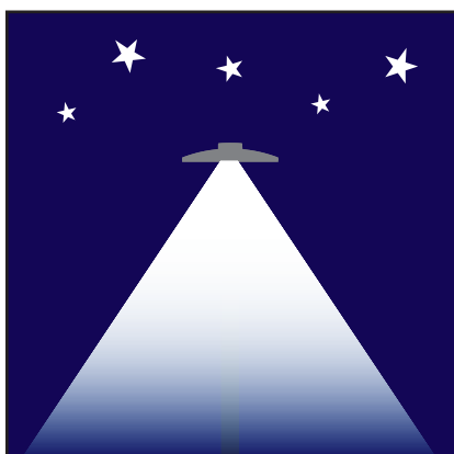
The CESP is a complete cutoff, fully shielded area light that minimizes glare, while reducing light trespass. (The maximum luminous beam angle 120°)
